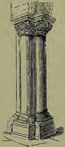
Fig. 1. Norman Clustered Pillar.
