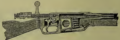
Fig. 4.—German Mauser Magazine Rifle, in section.
