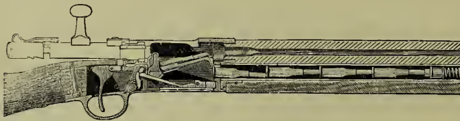
Fig. 3.—French Lebel Magazine Rifle, in section.
